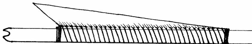
**Figure A1.5** Detail of a tie-down fletch (other fletches not shown for clarity). The fletch is securely tied down at each end, as well as along its length, with approximately 1/4" between windings.
