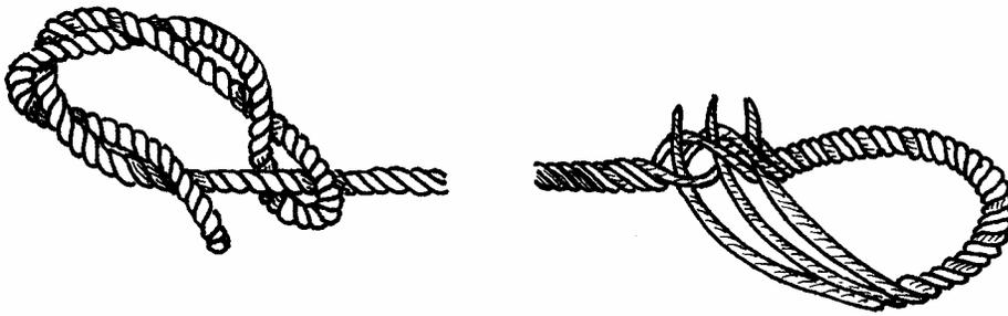
**Figure A1.2** The upper laid-in loop and bowyers knot used to attach the bowstring to the nocks on the bow.
